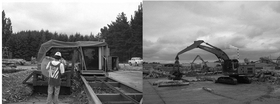
Figure 1 The Logmeister scanner (left) runs on rails parallel to the log and virtually bucks the stem. The bucked stem solution is wirelessly passed to a second machine (right) with a processor head which cuts the stems into logs.
